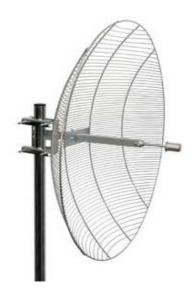
High-directional parabolic WLAN antenna working in 5 GHz band. Grid 32-5G v2 is assigned for extremely long links (over 20km). The antenna has excellent parameters and increased resistance against the opposite polarization. Grid 32-5G v2 has very good front to back performance. Its design ensures very good wind loading characteristics.
