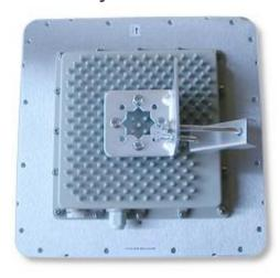
Assemble the L-Shaped Mounting bracket using the 4 screws already attached on the enclosure.
